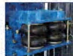
Mould Frame Damping Airbag:
